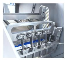
Machine designed for cutting frozen blocks up to -25C for cubes or slices by replaceable knives: main and transverse.
