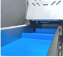
After cutting smaller pieces of the frozen product go directly into the trolley or on conveyer that transports them for further grinding and processing, usually with the help of machines such as grinder, cutter or mixer.
