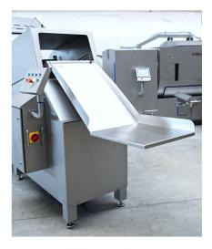
The blocks fall by gravity into the cutting zone with the help of manual, pneumatic or conveyer loader.
