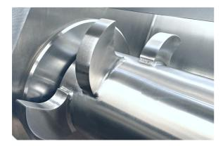
Crushing of the frozen blocks is executed with the help of slow speed, strong resistant, robust tooth head.
