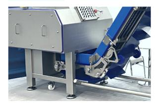
After cutting smaller pieces of the frozen product go directly into the trolley or on conveyer that transports them for further grinding and processing, usually with the help of machines such as grinder, cutter or mixer.
