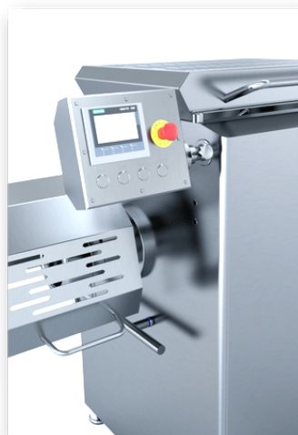
PLC control with touch screen
